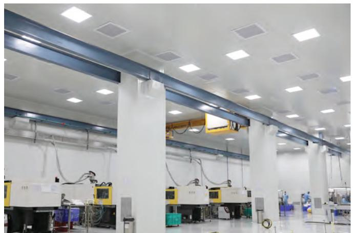
Facility validated from ISO CLASS 8 & equipped with latest robotics & automation machines
