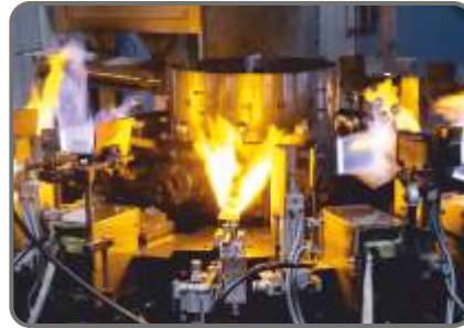
AUTOMATIC FLASK FORMING MACHINE : 800 pcs per shift
