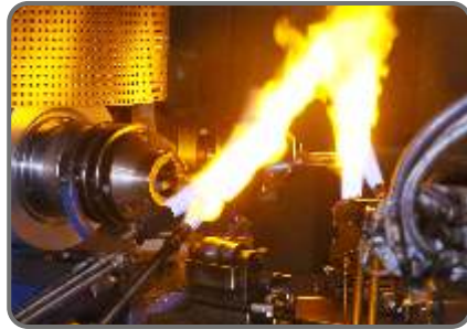
AUTOMATIC JOINT FORMING MACHINE : 2000 pcs per shift
